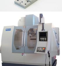
CNC machnining parameters:X: 1100 mm3D millingY: 650 mmPrecision: 10μmZ: 650 mm2
